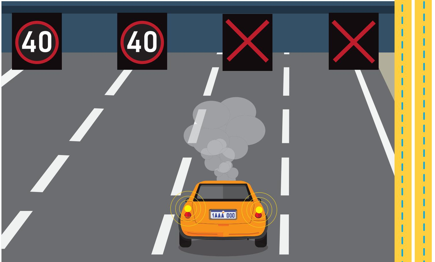
There are 12 overhead electronic sign structures on our new Smart Freeway, between the Mt Henry Bridge and the Narrows Bridge. These are designed to keep motorists informed, adjust speed limits and close lanes when needed, to help traffic flow more smoothly.
